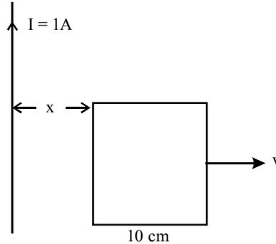
The e.m.f. induced at the time the left arm of the frame is at  $x = 10 \text{ cm}$  from the wire is:
